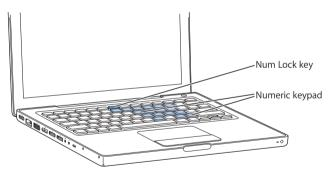
To use the numeric keypad, press the Num Lock key. An indicator light on the Num Lock key glows when the keypad is active. When you finish using the keypad, press the Num Lock key again to turn it off.
