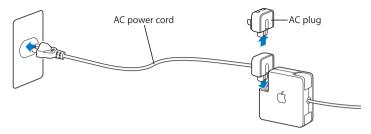
Use the AC power cord and connect it to a grounded power outlet when one is available. Use only the AC power cord that came with your power adapter. Make sure to push the power plug snugly into the power adapter port on the computer to ensure it is engaged and power is flowing to the computer. If the cord is plugged in properly, you'll see a glowing indicator light on the end of the cord that plugs into your MacBook.
