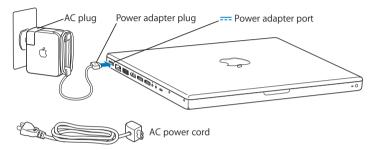
To extend the reach of your power adapter, you can attach the AC power cord. First pull up on the AC plug to remove it from the adapter, and then attach the included AC power cord to the adapter. Plug the other end into a power outlet. For an illustration, see page 31.
