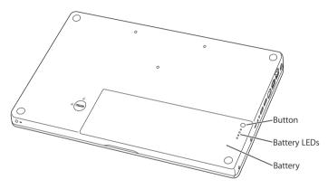
If the battery icon in the Finder menu bar is set to show the percentage of charge, sometimes the battery won't show a full 100 percent charge when the power adapter is attached. This is normal behavior; battery life is maximized if charging is not continuously cycled on and off when the battery's charge capacity is between 95 and 100 percent. When the battery level eventually drops below 95 percent, it will charge all the way up to 100 percent.
