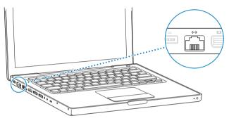
Connecting to a network gives you access to other computers and potentially to network printers, modems, email, and the Internet. You can use Ethernet to share files between two computers or set up a small network. The Ethernet port on your MacBook automatically detects other Ethernet devices. You don't need an Ethernet crossover cable when connecting to other Ethernet devices.
