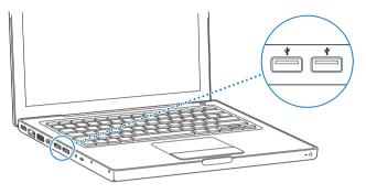
To use a USB device with your computer, connect the device to the computer. Your computer automatically detects newly connected devices and loads the correct software to work with the device.
